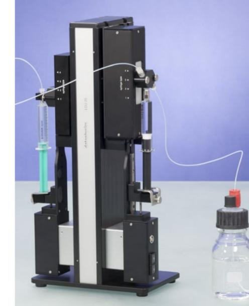
An **automatic, software-controlled liquid dosing and refill unit** can be used to create **sequential concentration series** of, for example, surfactant solutions. Hence, with a special software module the critical micelle concentration (**CMC**) can be determined in a series of experiments during which no manual user intervention is required.
